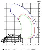
Working with outriggers, cage load 100 kg
